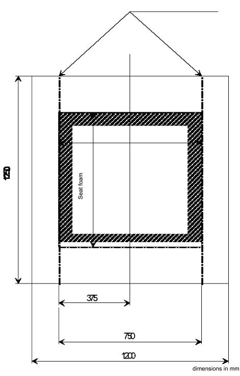
Figure 3: Dimensions of the cover material
