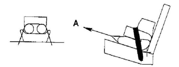
Figure 2: Booster pull test using manikin block
