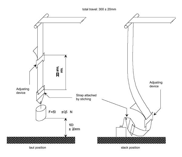
The load of 50 N on the testing device shall be vertically guided in such a way as to prevent load-swing and twisting of the strap.
