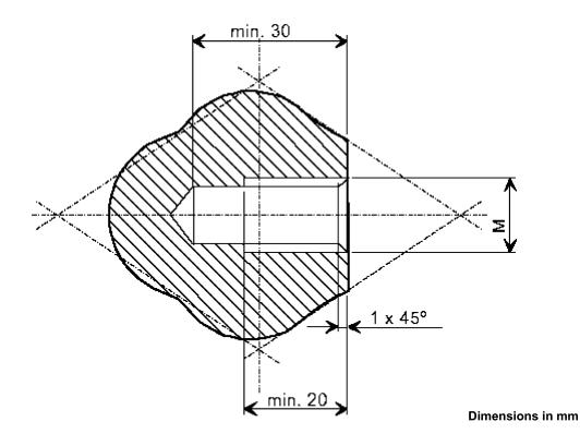
Figure 3: Stopping device olive-shaped knob
